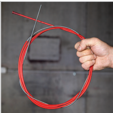
(4) Carefully unravel the new liner, avoiding creating any kinks in the liner.
