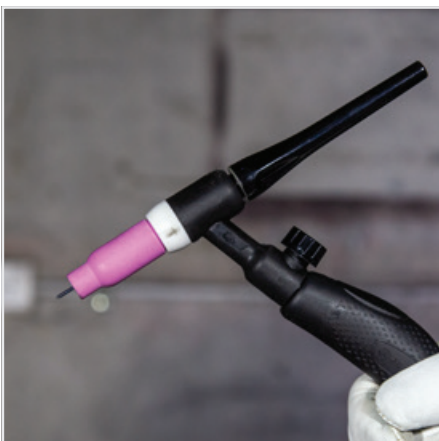
(6) Assemble front end parts of the TIG torch.
