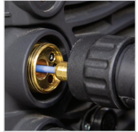
(12) Carefully feed the Polymide liner into the inlet guide tube hole of the torch Euro receptacle
