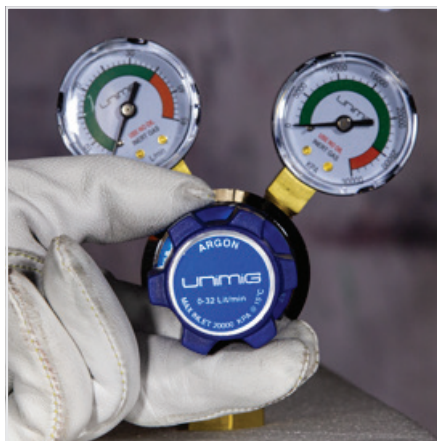
(7) Carefully open the valve of the gas cylinder, set the flow to 6-10 l/min
