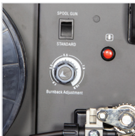
(16) Adjust the burn back control to prevent the wire sticking in the weld pool. Burn back control is located above the wire feed motor
