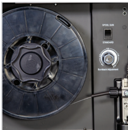
(7) Place wire onto spool holder - (spool retaining nut is left hand thread ) Feed the wire through the inlet guide tube into the drive roller.
