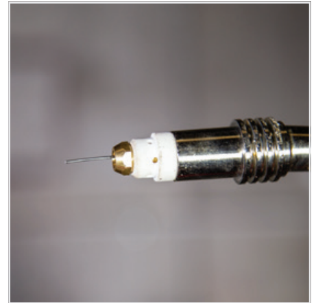
(11) Remove the gas nozzle and contact tip from the front end of the MIG torch.
