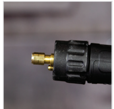
(6) Fit the liner retaining nut and screw only 1/2 way down.
